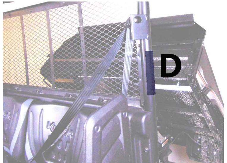
Figure 4: Shows placement of 8" strips D.
