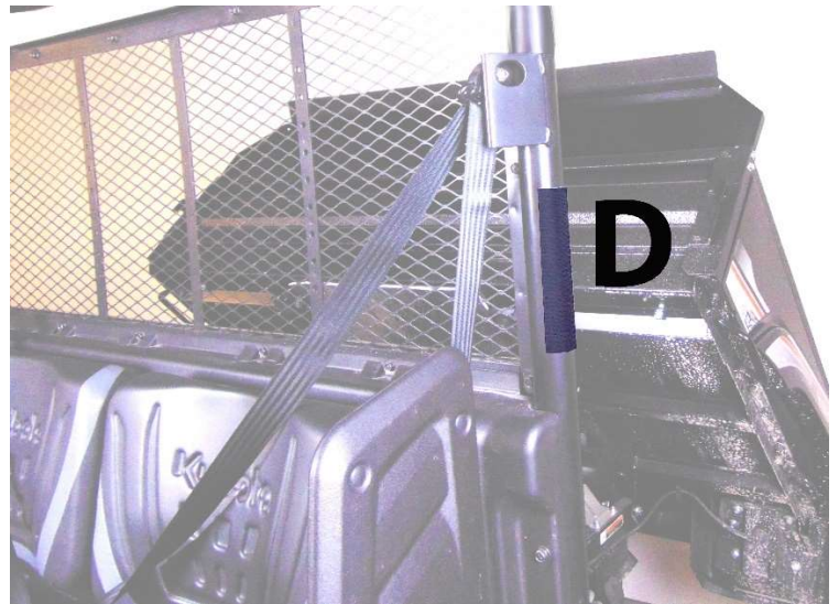
Figure 4: Shows placement of 8" strips D.
