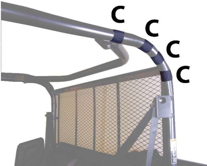
Figure 3: Shows position of 6" Velcro strips C. The double sided straps will wrap around these Velcro strips.
