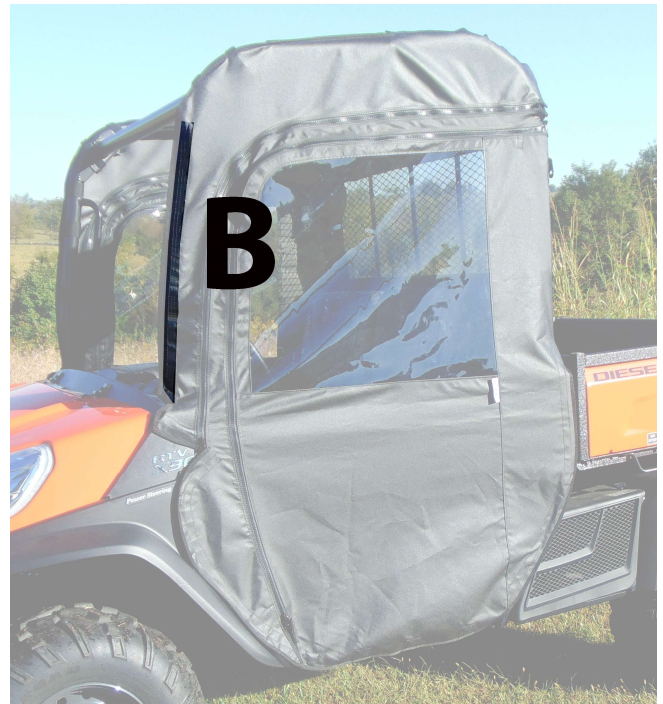
Figure 2: Velcro for tabs B is sewn on to the outside of the door.
