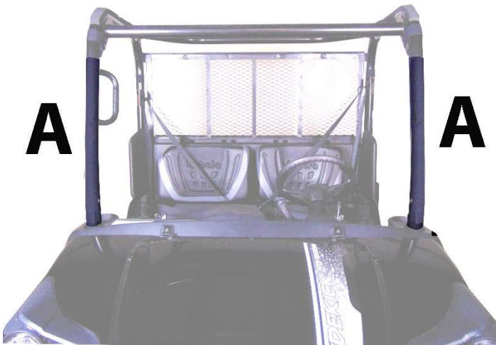
Figure 1: Shows placement of Velcro strip A.
