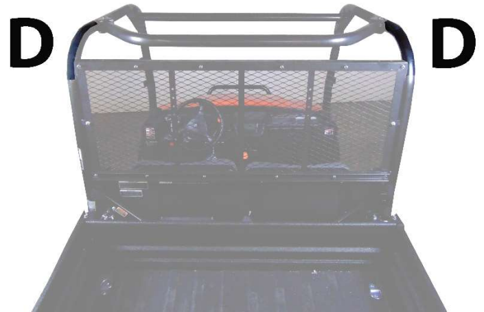
Figure 4: Shows placement of Velcro strips D.
