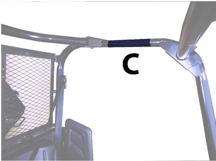
Figure 1: Shows placement of Velcro strips C.
