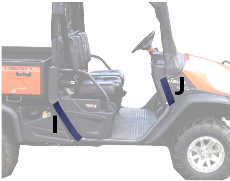
Figure 7: Shows position of 15" and 10" Velcro strips I and J you will place identical strips on the drivers side.
