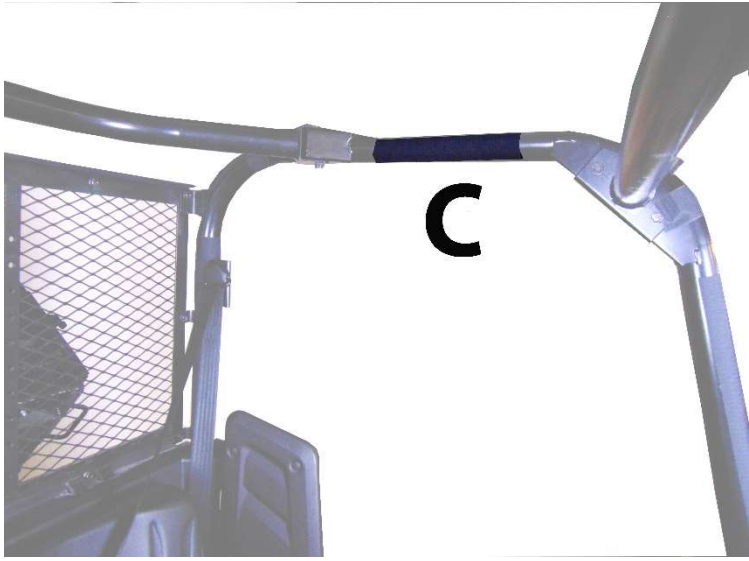
Figure 1: Shows placement of Velcro strips C.
