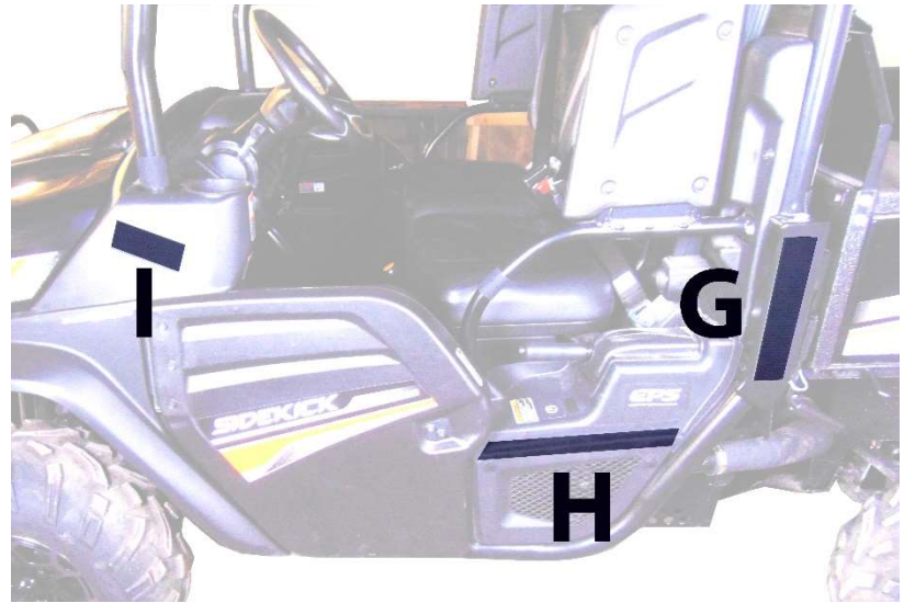
Figure 6: Shows position of Velcro strips G, H, and I. You will position identical strips on the driver's side.
