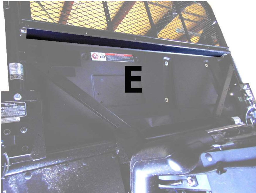
Figure 5: Shows position of Velcro strip E. Raise bed and place beneath the factory grate. The bottom of the back panel will fold around to the flat area beneath the grate.
