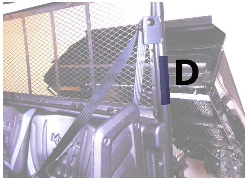
Figure 4: Shows placement of 8" strips D.
