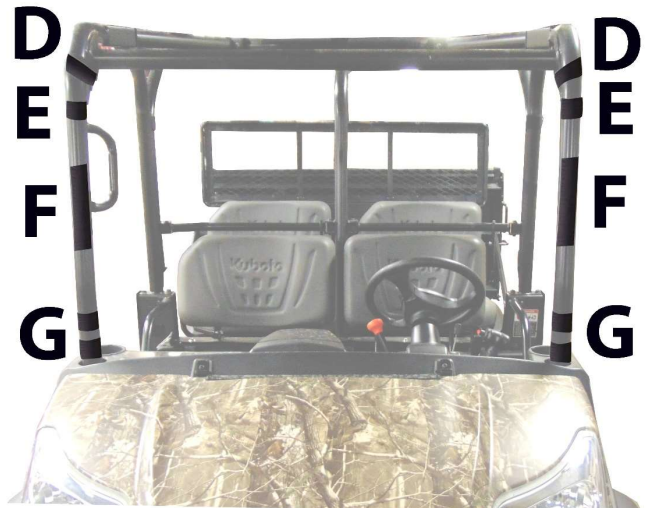
Figure 2: Tabs wrap around the front of the roll bars and attach to adhesive strips, D and G (double sided straps) wrap around adhesive Velcro.
