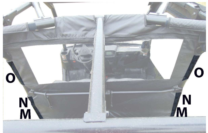
Figure 4: Velcro sewn on back panel for tabs on the back of the door.
