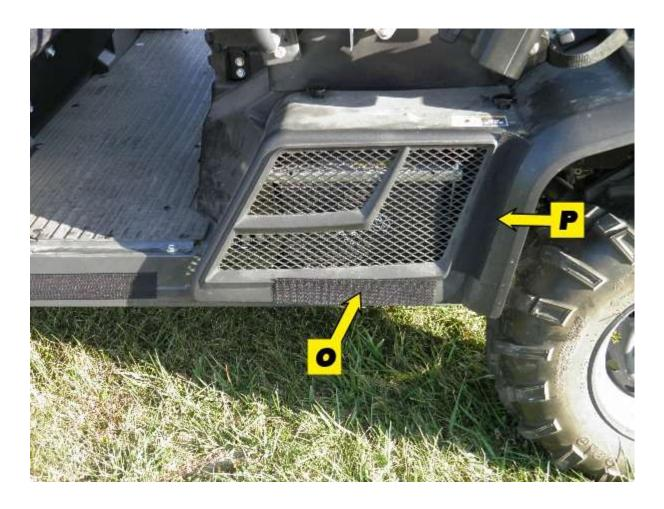
**Step 5:** Begin attaching the adhesive hook strips for the front door panels as indicated below. If necessary, hold the door panels to the roll cage and note the locations of the sewn-in loop and double-sided straps. The sewn-in loop along the back side of the front door panels attach to the exposed hook sewn on the outside of the rear door panels. Again, the door panels should hang just to the bottom of the rocker panel area.
