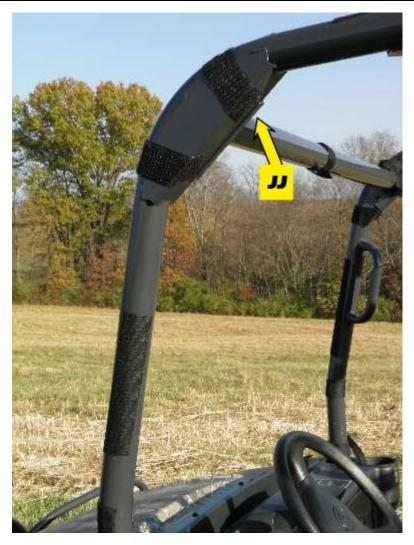
**Step 7**: Repeat any steps necessary to achieve a snug fit on the cab frame.
