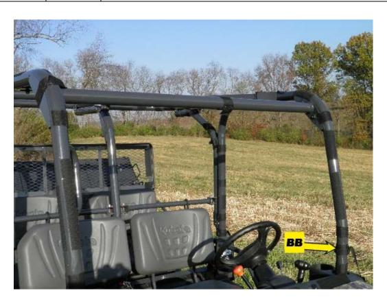
Wrap horizontally around the bottom of the middle roll bars. Wrap
