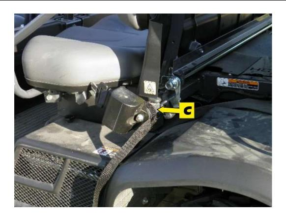
Attach horizontally to the small bar behind the back seats. Attach the sewn-in loop along the bottom of the rear panel to the adhesive hook strips.
