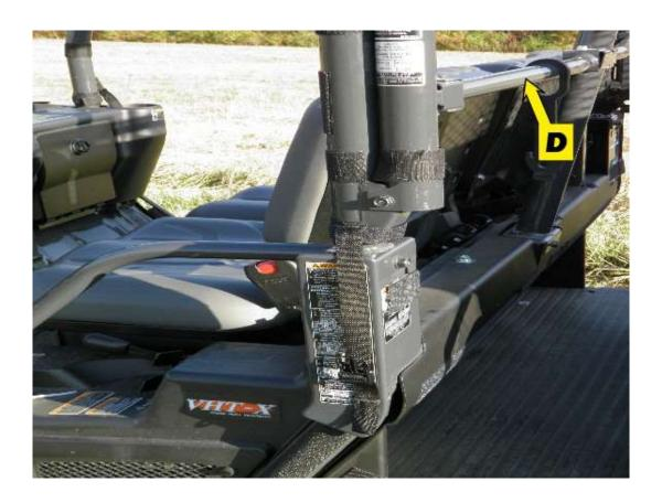
**Step 4:** Attach the rear door panels before attaching the front door panels. Again, hold the panel to the roll cage and note the locations of the sewn-in loop. Repeat as needed for location assistance. The door panels should hang so that the bottom of the door panels come to the bottom of the rocker panel area. Attach the adhesive hook strips as indicated below.
