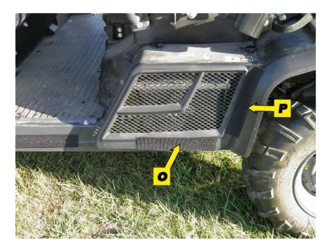
**Step 4:** Begin attaching the adhesive hook strips for the front door panels as indicated below. If necessary, hold the door panels to the roll cage and note the locations of the sewn-in loop and double-sided straps. The sewn-in loop along the back side of the front door panels attach to the exposed hook sewn on the outside of the rear door panels. Again, the door panels should hang just to the bottom of the rocker panel area.
