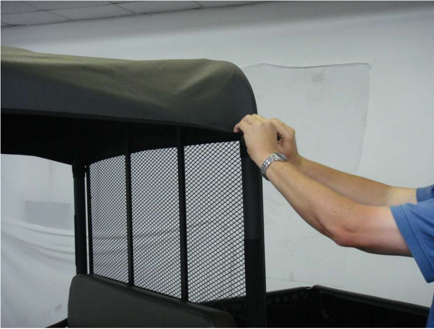
Figure 5.1 – Pull down firmly and attach rear Velcro Tabs to installed Velcro strips
