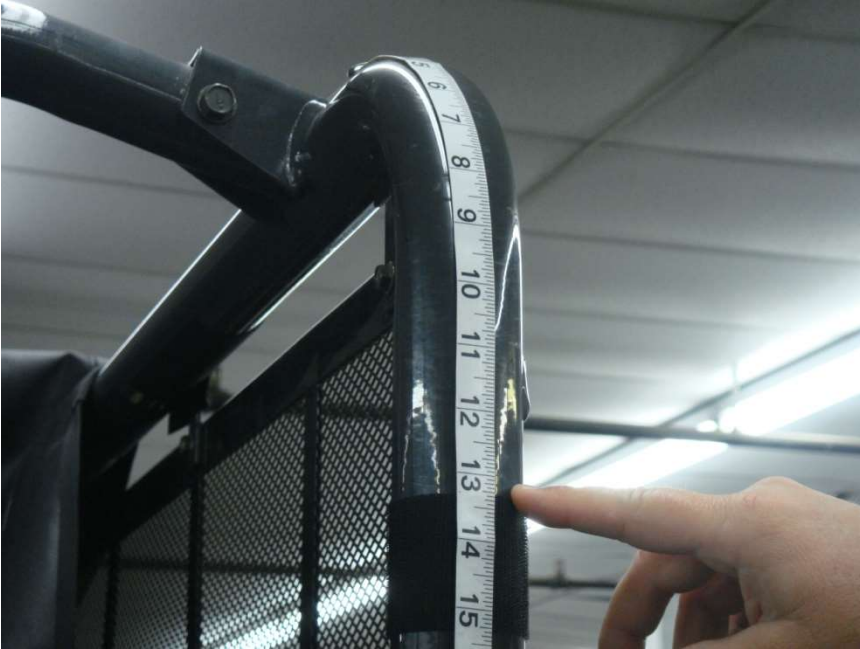
Figure 3.1 – Place Rear Velcro strips 13 1/4 inches below the top roll bar cross member brackets located at the top of the Cab Roll Bar Structure
