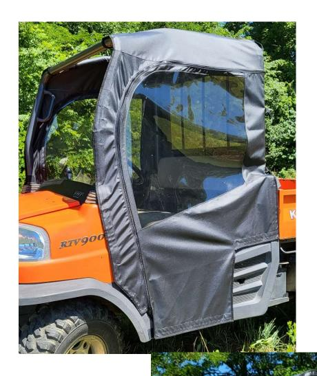
The top of the door kit has a strap that should be installed under the back panel. Pull back the back panel and wrap the strap around the roll bar. Then reattach the back panel.
