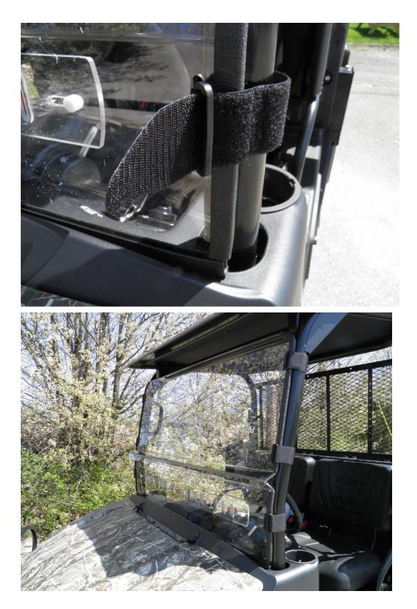
**Step 7:** Repeat Step 4 for each of the strap slots in the upper windshield section.
