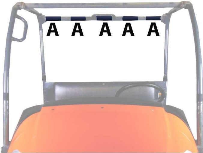
Figure 1: Shows position of 24" Velcro strip A. Wrap tab over the top of the roll bar and attach to the adhesive Velcro strip.
