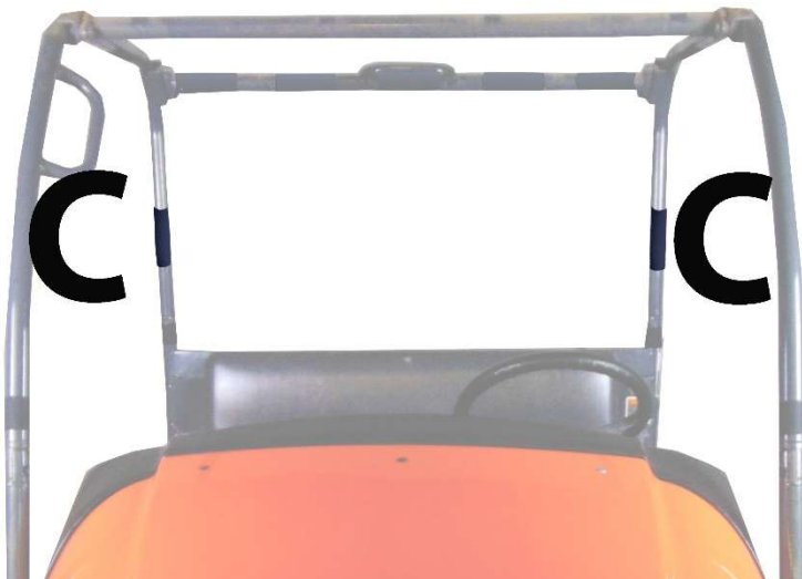
Figure 3: Shows position of 6" Velcro strips C. The double sided straps will wrap around these Velcro strips.
