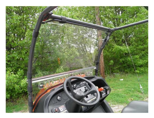
**Step 6:** Adjust the straps as needed to align the windshield.
