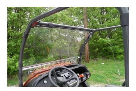
**Step 11:** Adjust the straps as needed to align the windshield.
