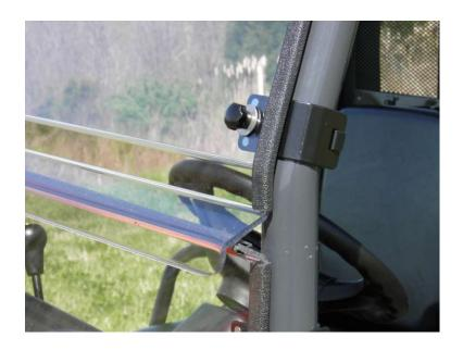
**Step 5:** When satisfied that the bottom windshield section is positioned properly, tighten the two clamps nuts on each clamp.
