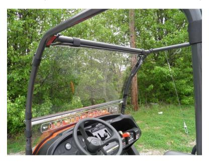
**Step 9:** When satisfied that the upper windshield section is positioned properly, tighten the two clamps nuts on each clamp.
