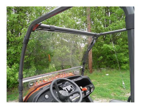
**Step 7:** When satisfied that the upper windshield section is positioned properly, tighten the nuts on each clamp.
