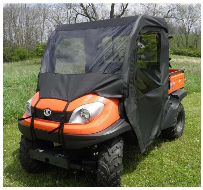
When all straps are attached walk around the UTV pulling your tension straps down to tighten the windshield top over the door and rear window.
