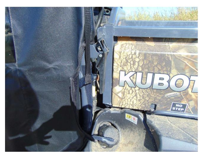
Attach double sided strap to the prepositioned Velcro, wrap straps around the roll bar below the seat rest bar.
