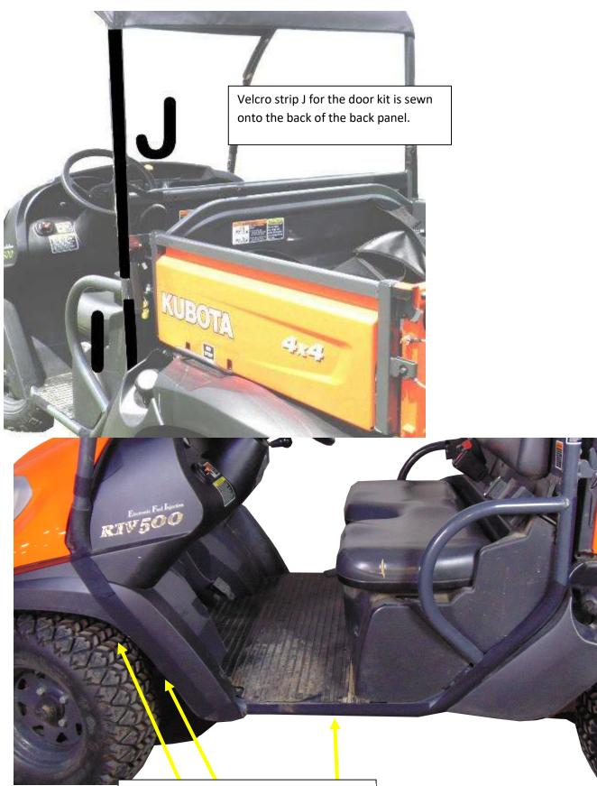
TABS D AND E ADHESIVE HOOK STRIPS WILL ATTACH TO THE INSIDE OF THE WHEEL WELL, STRIP F WILL ATTACH BENEATH THE "FLOOR" ROLL BAR.
