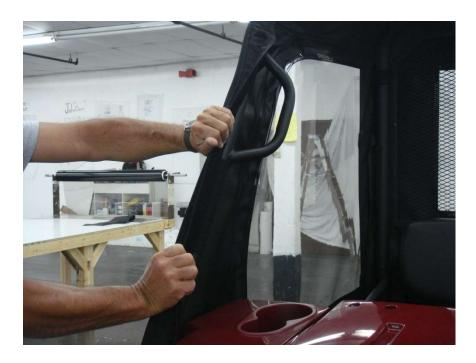
**Step 6:** The webbing/Velcro strip that runs the length of the front roll bars will need to be cut to accommodate the windshield clamps and the grab handle. With chalk, mark the webbing strip where cuts will be made. **DO NOT CUT INTO THE BINDING.**
