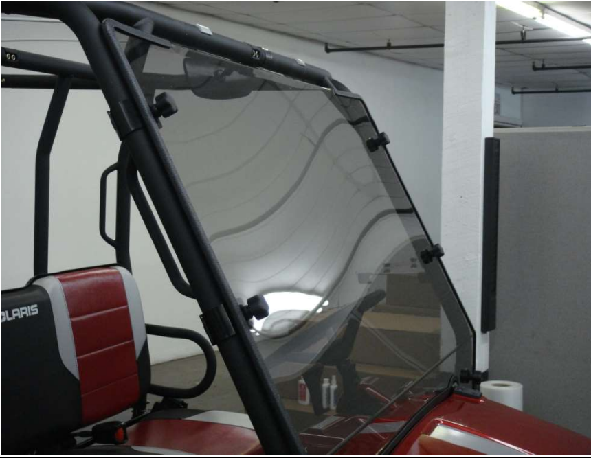
Figure 3.2 - place clamps at appropriate locations on the front Roll Bar uprights to match the windshield's holes.
