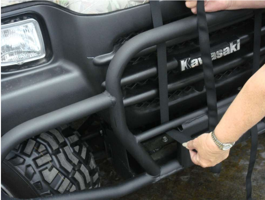
Figure 4.1 - run front hood straps through the center bar of the front bumper
