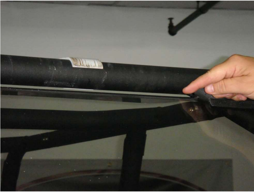
Figure 2.3 - place windshield so that the top polycarbonate tab is approx ½" below the Top Roll Bar Cross-member
