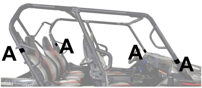
When installing a top cap with a full cab and a windshield, the top caps double sided straps will set underneath the windshield and door kit. You may choose to cut a space in the previously installed Velcro to install Velcro that will wrap around the roll bar.
