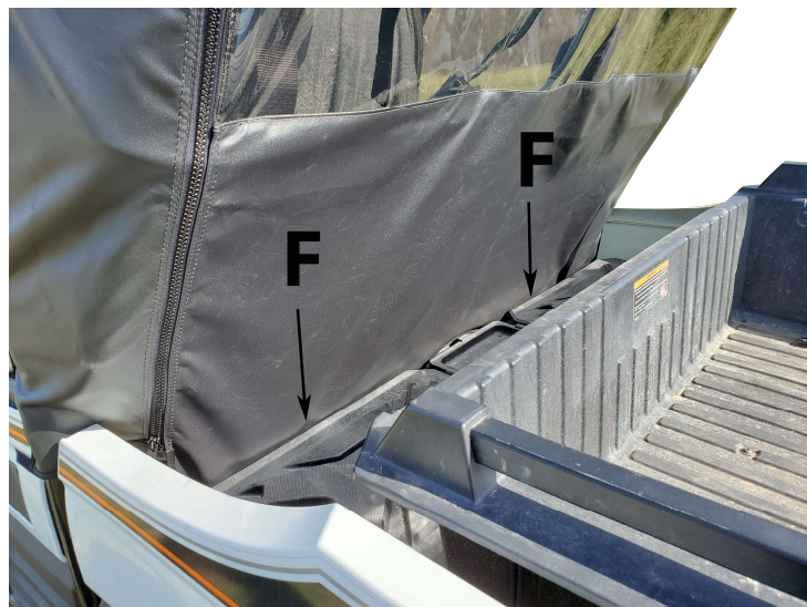
Figure 4: Pull your back panel down tight and stick the bottom to these strips.
