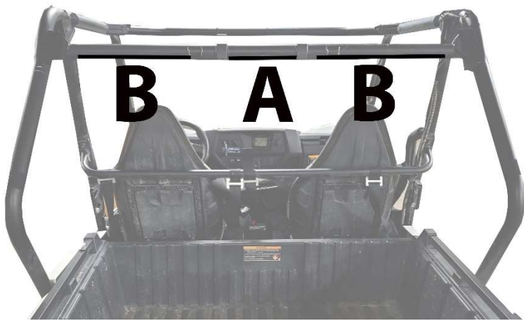
Figure 1: Pull your back panel from the inside and wrap the top of the back panel over the rear roll bar and around to the outside. More photos below.
