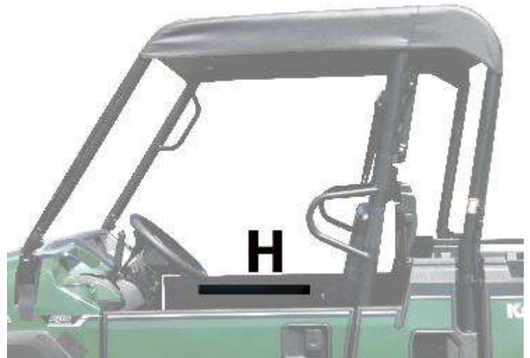
Figure 6: Peel off white backing on magnet strip and stick to inside of the factory half door.
