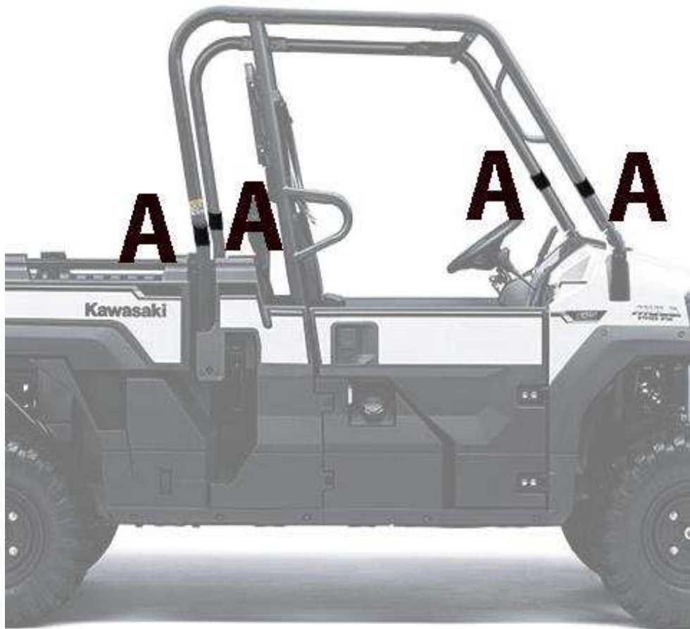
Figure 1: WRAP THESE VELCRO STRIPS AROUND THE ROLL BAR ON EITHER SIDE OF THE MACHINE AND ATTACH DOUBLE-SIDED STRAP.
