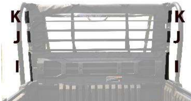
Figure 7: Photo shows the location of the adhesive Velcro on the back roll bars. These strips will be sewn on to the back panel.
