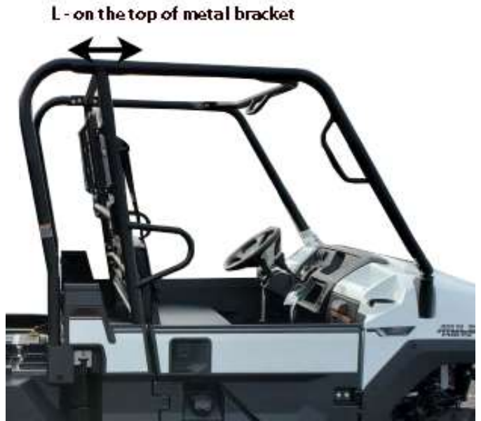
Figure 6: Shows position of Velcro strip L. Place on the top of the metal bracket and pull tab up and over to meet the strip.
