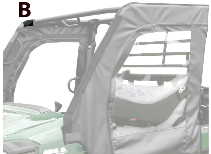
Figure 2: Shows placement of 4" Velcro strips B. Tab B will also go up and around the top roll bar and attach to adhesive strip.
