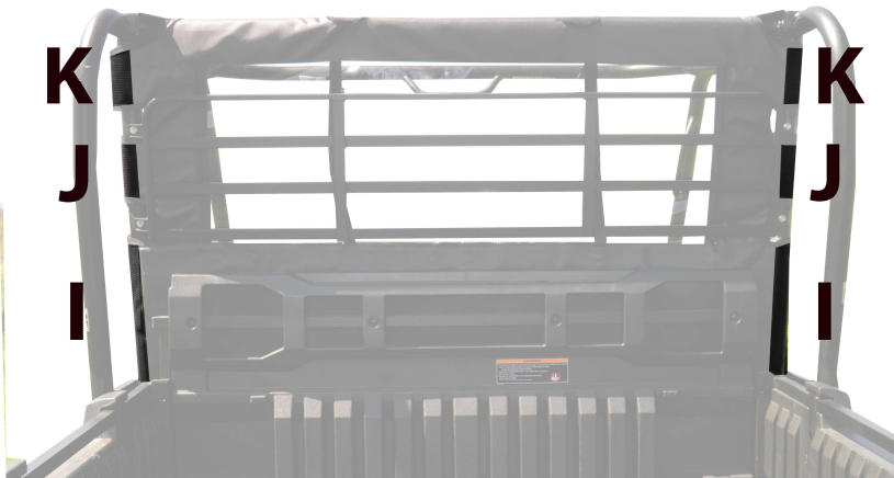
Figure 5: Photo shows Velcro sewn on the back panel. The door kit will have Velcro tabs that attach to the back panel.
