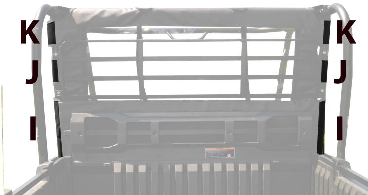
Figure 7: Photo shows the location of the adhesive Velcro on the back roll bars.
