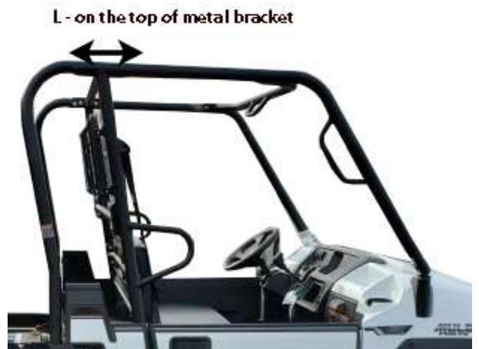
Figure 8: Shows position of Velcro strip L. Place on the top of the metal bracket and pull tab up and over to meet the strip.
