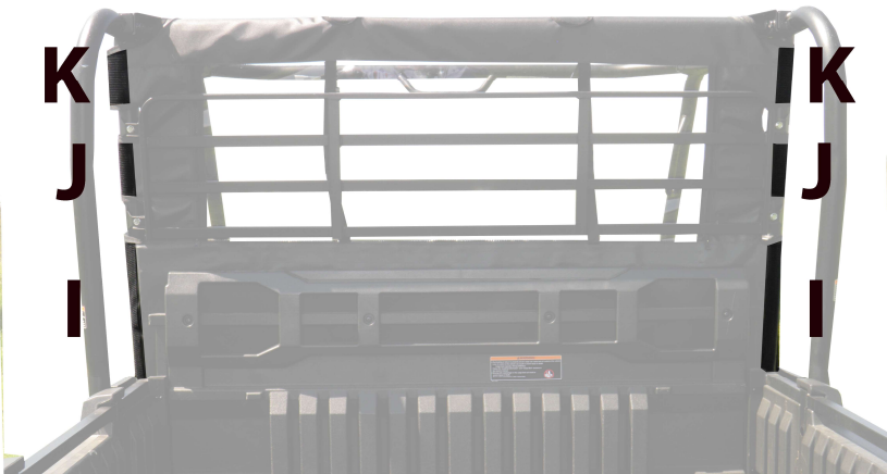
Figure 5: Photo shows the location of the adhesive Velcro.
