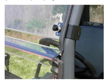
**Step 3: 2" QUICK CONNECT CLAMPS ARE USED TO SECURE THE WINDSHIELD IN PLACE.** One at a time, attach a clamp to the front roll bars corresponding to the pre-routed openings in the lower windshield section. The flat side of the clamps
