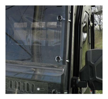
**Step 4:** When satisfied that the bottom windshield section is positioned properly, tighten the nuts on each clamp.
