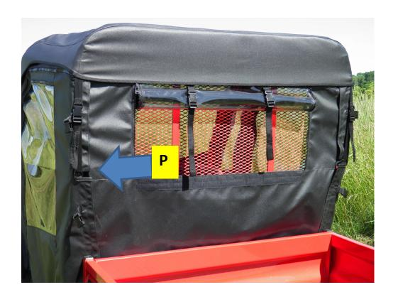
The buckle straps in the back are installed by wrapping the end of the straps around the rollbar underneath the back panel and door kit. Insert the end of the straps through the cut outs made in the back panel and door kit. Then connect the buckles.
