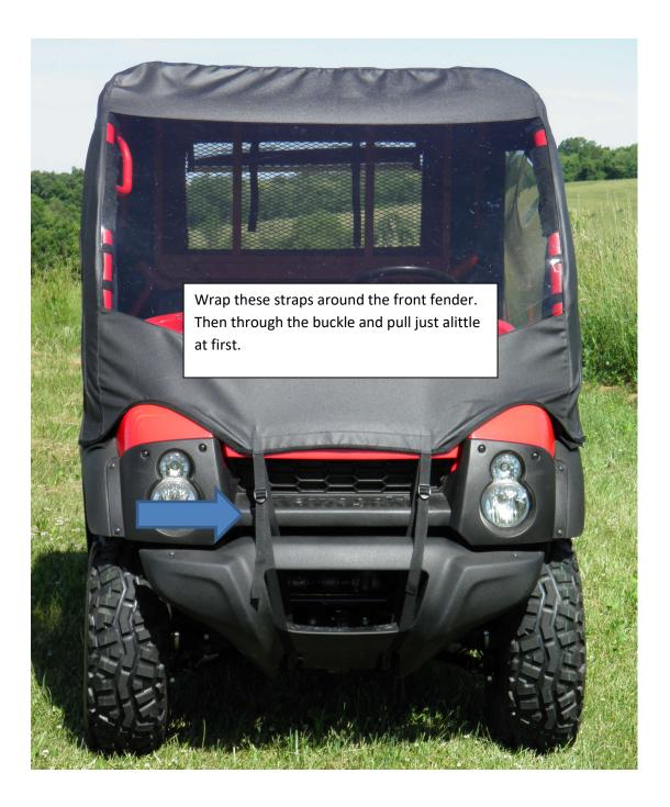
After you have attach the front buckles, work your way around the UTV tightening all the straps. You need to make more than one trip around to get every thing pulled tight and even.
