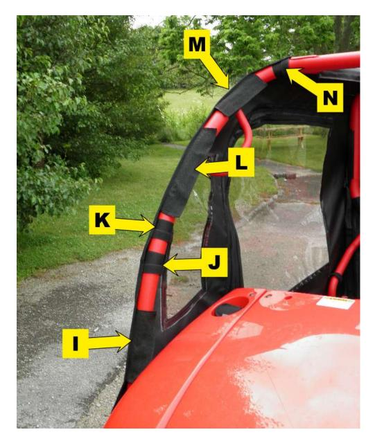
**Step 4:** After all adhesive hook strips are attached, begin attaching the enclosure to the cab frame. As you attach the hook and loop, square each panel to the frame. **PLEASE NOTE, FOR MAXIMUM ADHESION, ALLOW THE ADHESIVE HOOK TO ADHERE TO THE FRAME FOR 24 HOURS BEFORE PULLING AGAINST THE HOOK WITH THE LOOP STRIPS.**
