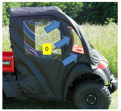
Arrows point to the 8 inch tabs sewn on the inside of the windshield top. Velcro for these tabs are sewn on to the outside of the door kit. Attach the tabs to the Velcro sewn on the door kit.
