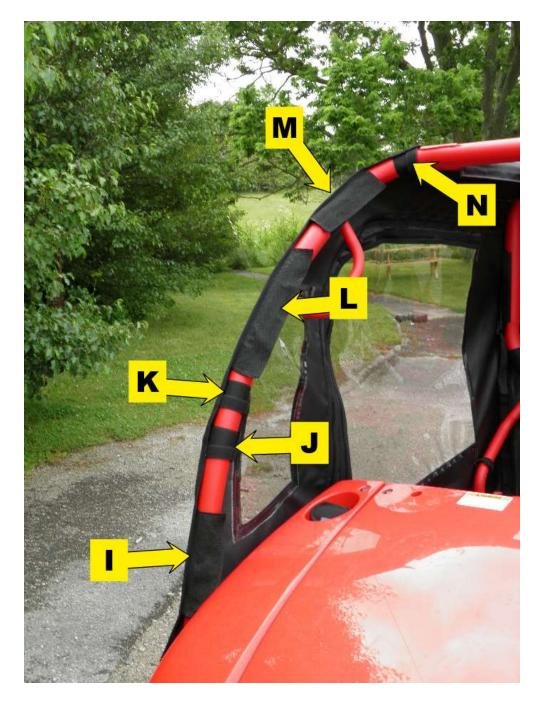
**Step 4:** After all adhesive hook strips are attached, begin attaching the enclosure to the cab frame. As you attach the hook and loop, square each panel to the frame. **PLEASE NOTE, FOR MAXIMUM ADHESION, ALLOW THE ADHESIVE HOOK TO ADHERE TO THE FRAME FOR 24 HOURS BEFORE PULLING AGAINST THE HOOK WITH THE LOOP STRIPS.**
