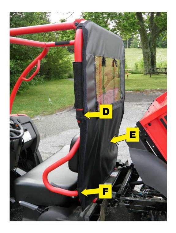
**Step 3:** After all adhesive hook strips are attached, begin attaching the enclosure to the cab frame. As you attach the hook and loop, square each panel to the frame. **PLEASE NOTE, FOR MAXIMUM ADHESION, ALLOW THE ADHESIVE HOOK TO ADHERE TO THE FRAME FOR 24 HOURS BEFORE PULLING AGAINST THE HOOK WITH THE LOOP STRIPS.**
