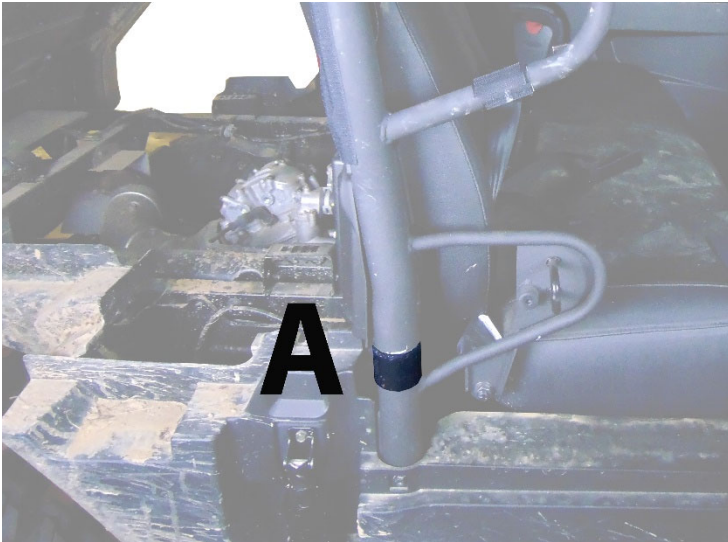
Figure 1: RAISE THE BED, WRAP THESE VELCRO STRIPS AROUND THE ROLL BAR ON EITHER SIDE OF THE MACHINE AND ATTACH DOUBLE-SIDED STRAP.
