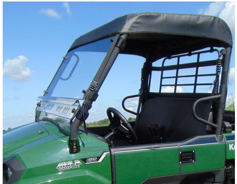
Figure 1: WE HAVE SEWN DOUBLE SIDED STRAPS ON TO THE BACK OF THE TOP CAP TO LOOP AROUND THE TOP OF THE METAL GRATE ON THE BACK OF THE MACHINE. LOOPING THESE STRAPS WILL PREVENT THE TOPCAP FROM MOVING IN THE WIND.
