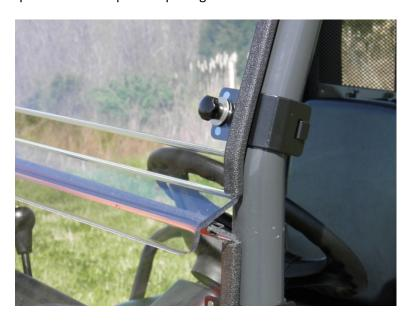
Step 3: 2" QUICK CONNECT CLAMPS (with velcro strips) ARE USED TO SECURE THE WINDSHIELD IN PLACE. One at a time, peel the adhesive backing from the velcro strips and place them attach a clamp to the front roll bars corresponding to the pre-routed openings in the lower windshield section. The flat side of the clamps should face the windshield when installed properly. Tighten the nuts on the clamps enough to hold them in place, but allowing movement up and down for proper positioning.
