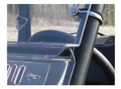
**Step 4:** When satisfied that the bottom windshield section is positioned properly, tighten the nuts on each clamp.
