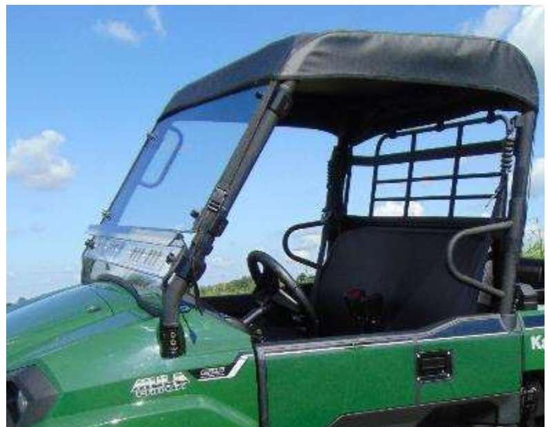
Figure 3: WE HAVE SEWN DOUBLE SIDED STRAPS ON TO THE BACK OF THE TOP CAP TO LOOP AROUND THE TOP OF THE METAL GRATE ON THE BACK OF THE MACHINE. DO NOT USE WITH REAR PANEL.
