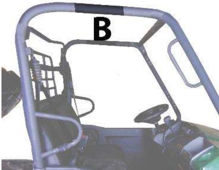
Figure 2: ATTACH THESE STRIPS HORIZONTALLY TO THE OUTSIDE EDGE OF THE TOP SIDE ROLL BAR. STRETCH THE TAB AROUND THE TOP AND PULL TIGHT TO FLATTEN OUT THE ROOF OF THE TOP CAP. DO NOT USE WITH DOOR KIT.
