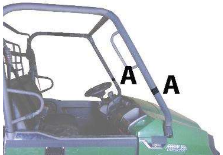
Figure2: WRAP THESE VELCRO STRIPS AROUND THE ROLL BAR AND ATTACH DOUBLE-SIDED STRAPS.
