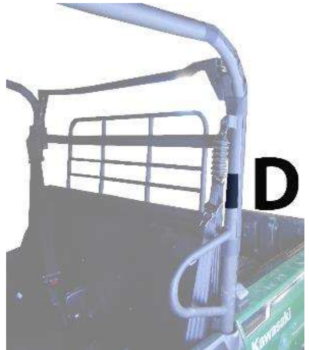
Figure 4: Shows placement of 6" strips D.
