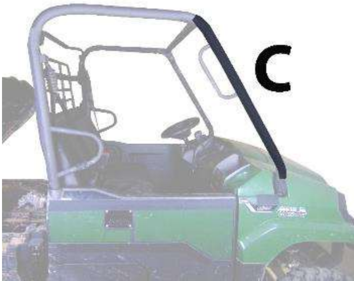
Figure 1: Shows placement of 38" Velcro strips C. The tabs on the front of your doors will wrap around the front of the roll bar and attach to the Velcro strip, as well as the sewn in Velcro strip on the inside of the door.
