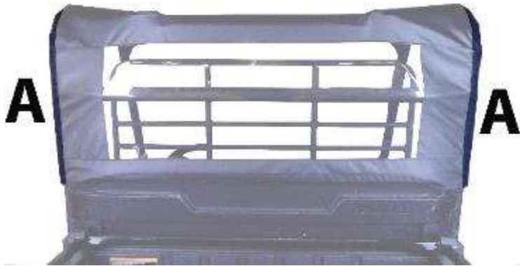
Figure 1: Shows placement of 27" Velcro strip A. Down the back of the roll bar.
