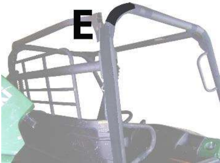
Figure 5: Photo shows placement of 7" Velcro strip E. The flap on the top of the rear door panel will "flap" over and stick to this strip.
