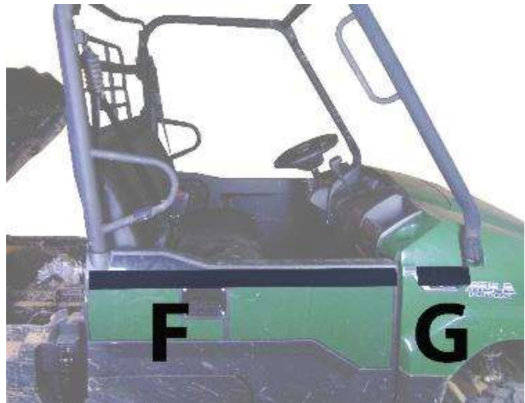
Figure 6: Shows position of 34" and 8" Velcro strips F and G.
