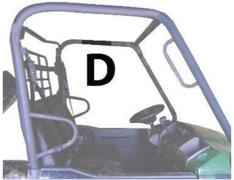
Figure 4: Shows placement of 12" Velcro strips D. This strip faces the inside of the cab. Wrap the tab over the top and attach to strip.
