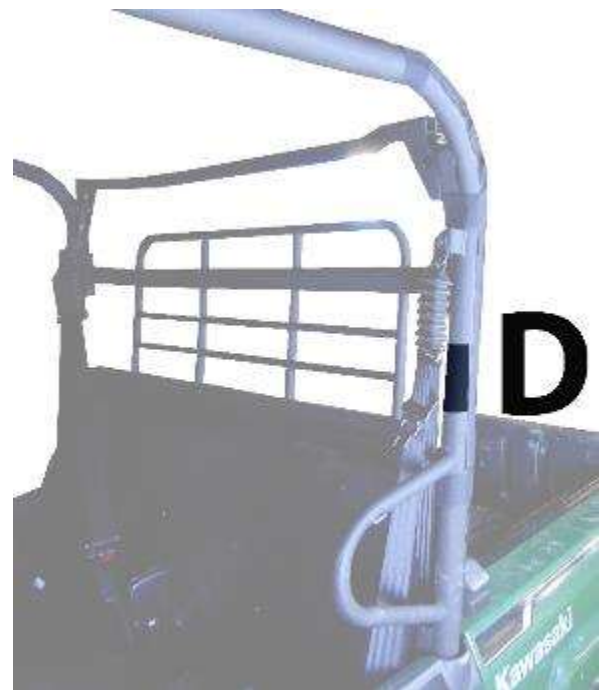
Figure 4: Shows placement of 6" strips D.
