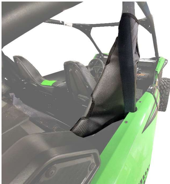
IF INSTALLED CORRECTLY YOUR SIDE PANELS SHOULD RESEMBLE THE PHOTO.
