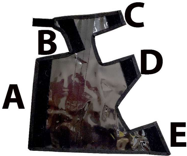
SIDE PANELS WILL NEED ADHESIVE VELCRO TO ATTACH TO ROLL BARS. YOU WILL PLACE SIDE PANELS ON EITHER SIDE OF THE UTV.
