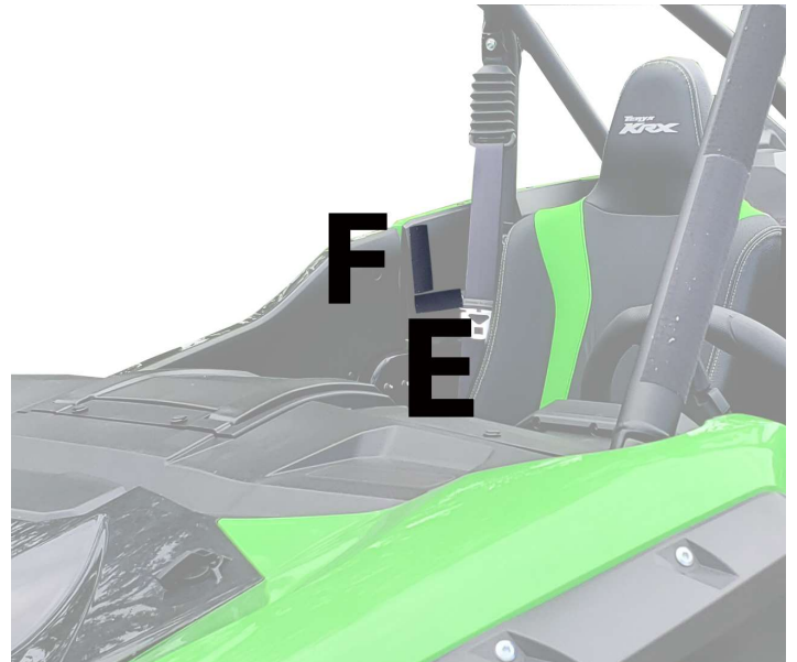
Figure 4: STRIPS E AND F ARE POSITIONED ON THE INSIDE OF THE UTV. NEAR THE DOOR LATCH.
