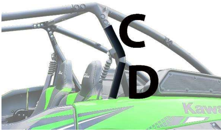
Figure 3: Pull back panel tight around the sides and attach.
