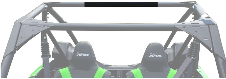
Figure 1: Wrap the top of the back panel around the top of the roll bar and attach.
