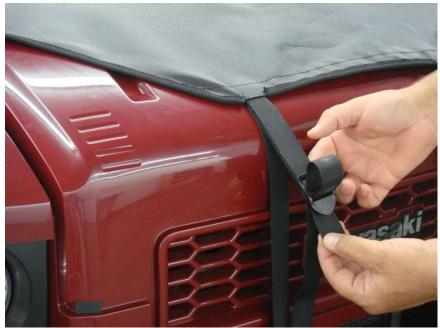
**Step 7**: Repeat any steps necessary to achieve a snug fit on the cab frame.
