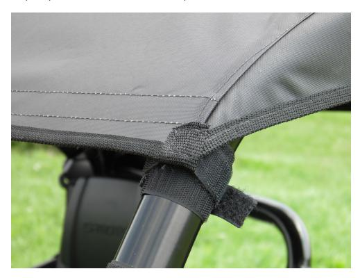
Step 5: If needed, grasp the webbing/loop tabs at the side seams and pull the top tight from side to side.
