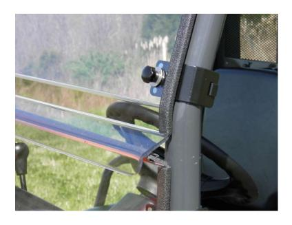
**Step 5:** When satisfied that the bottom windshield section is positioned properly, tighten the two clamps nuts on each clamp.
